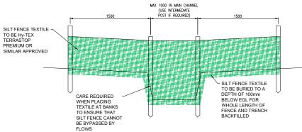
ELEVATION ON SILT FENCE AT DRAINAGE CHANNEL
